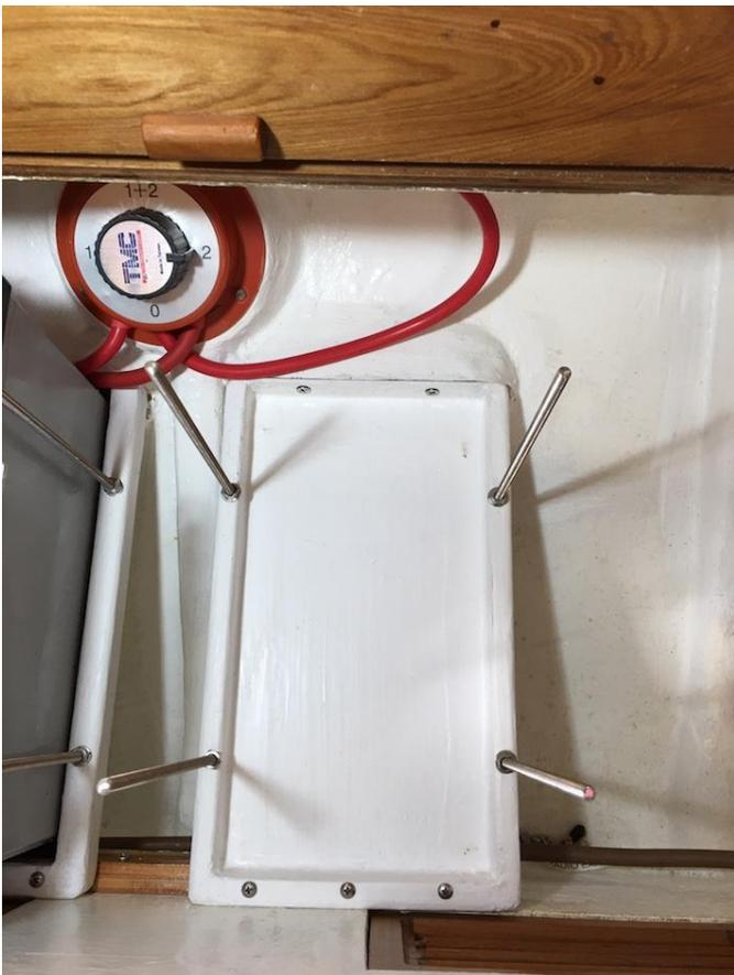
*The tray then finished off, gel coated and remounted into its original position under a bunk seat. Incidentally the four threaded rods hold a timber clamp to the top of the battery. The change-over switch allows for two different types of batteries to be used within the bank if one was ever so ldaft or so disposed.*
