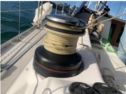
Winches do not see what is going on with the lines so it is imperative that one keeps their eyes on the winch as well as what the sheet is attached to.
